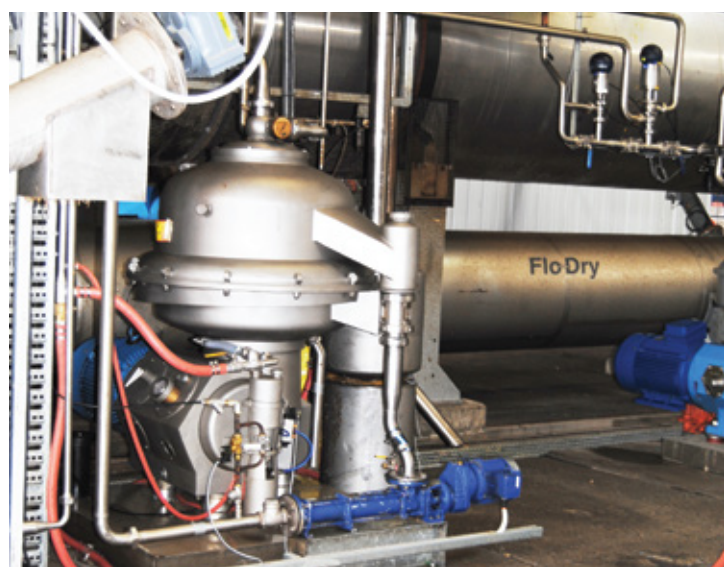
The gas-powered heart of the Wingfield plant... the rotary Flo Dry dryer (background) and a G Tech separator (foreground).
